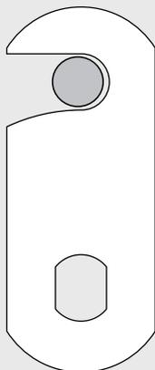
To order, measure from the centre of the mounting hole to the hook, and the tip of the cam.
