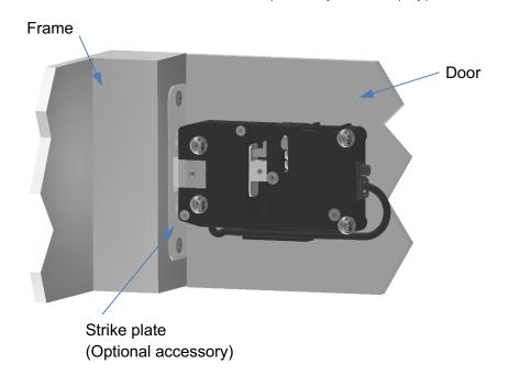
The latch and actuator should be fitted using 4mm fixings see drawings below for fixing positions. Same dimensions apply with and without door monitoring addition.
