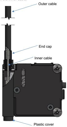
If you need to cut the cable to length, make sure you have suitable cutters, there are specific cutters that are suitable for Bowden cable. The inner cable should be approximately 60mm longer than the outer cable.
