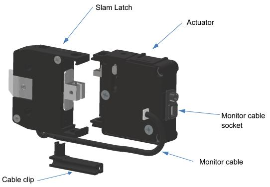
Plug the monitor cable (if fitted) into the socket on the back of the actuator. Push the cable clip in the hole at the bottom of the unit then feed the monitor cable into the slot.
