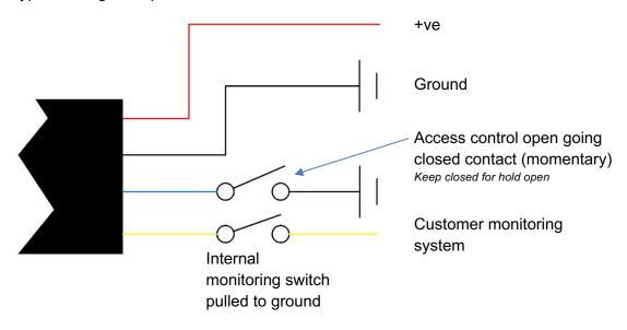
Check the operation of the lock electronically.
