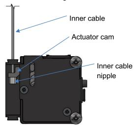
Fit plastic cover over actuator and inner cable. Insert end cap on to outer cable, then slide over the inner cable.
