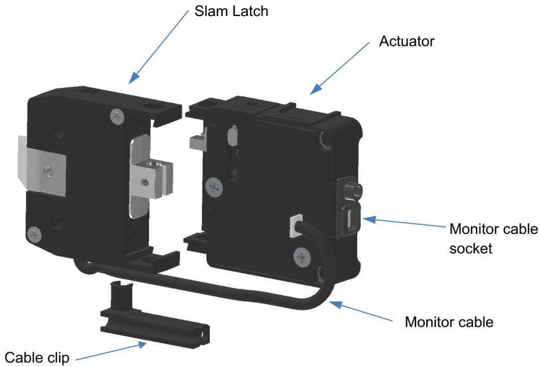
Plug the monitor cable (if fitted) into the socket on the back of the actuator. Push the cable clip in the hole at the bottom of the unit then feed the monitor cable into the slot.
